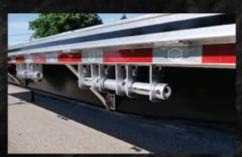
Load securement: J-track in floor, chain tie downs, or double LL winch track with galvanized winches
